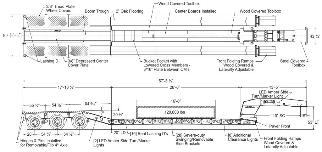
[12] - 275/70R22.5(H) Tubeless Radial Tires All Air Ride Suspensions with Mechanical Height Control Airlift on 3<sup>rd</sup> axle
