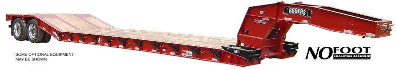
The ROGERS® ULTIMA™ Series CR35GR - The most versatile 35-ton capacity trailer combines extra easy loading with a spacious deck. Its capability to carry several machines on one trip makes this trailer especially well suited for customers in the paving industry. This trailer features the efficient No Foot® detachable gooseneck, the Croucher® low tapered front with a variety of ramp options, and the unique Gentle Riser™ transition from the deck to the rear frame for easy loading access.
