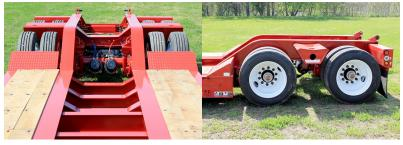
The use of high strength steel and superior manufacturing techniques are the hallmarks of ROGERS trailers durability. Main and side beams are fabricated of 100,000 psi steel and the frames are assembled with full-width cross members that are pierced through the main beam webs for maximum structural strength. The maximum depth "Bucket Pocket" gives the lowest loading profile available for loading excavators on the platform deck. Sloped 30° bridge ramps give easy access to the rear frame.
