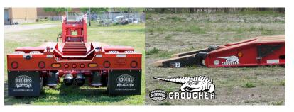
Lowered cross members in the rear frame form a "Boom Trough" which allows excavators to be hauled as low as possible. The ULTIMA Series CR40 includes air ride suspension, LED light package, and preparations for an optional removable 3rd axle. LED strobe lights with shut-off switch are also standard equipment. The **Croucher®** frame front is tapered top and bottom for an optimal load angle. A variety of ramp options are available to best suit your loading needs and preferences.
