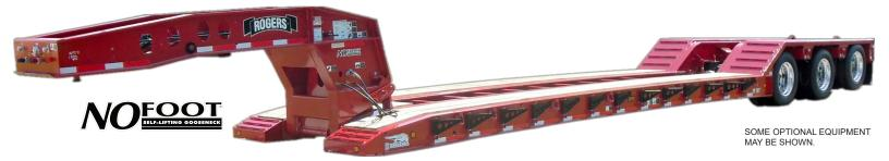
The ROGERS® ULTIMA™ Series SP55 - Aggressively designed to reduce weight without sacrificing performance, the ROGERS model SP55 is our latest 55-ton detachable gooseneck trailer. It features the **No Foot**® self-lifting gooseneck, the **Croucher**® low, tapered front end, and a "Bucket Pocket" in the deck. The wide "Boom Trough" in the trailer's rear frame combines with the 20" loaded deck height for a remarkably low transport height.
