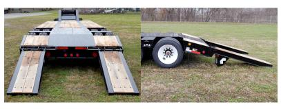
"E-Z Flip" loading ramps with 36" beavertail at 14° **slope:** These ramps are constructed from 50,000 psi minimum yield high strength steel, yet are light enough for easy operation. Dual springs assist lifting the ramps off the ground as well as off the deck, and they can be easily adjusted laterally to allow accomodate machines of various widths. Available in standard oak-covered or optional ladder style.
