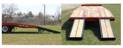
**Extra-long loading ramps with 72" beavertail at 8° slope:** Constructed from high-strength 50,000 psi minimum yield steel, these ramps are strong and durable yet lightweight for easy operation. Dual springs assist the operator lifting the ramps off the ground as well as off the deck. The ramps can be easily adjusted laterally to handle machines of various widths. Extra length reduces the climb angle for safer loading. These "E-Z Flip" ramps are standard oak-covered or optional ladder style.
