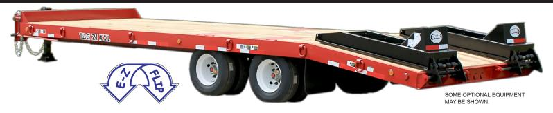
**ROGERS**® has two 21-ton models in the Tag-Along Series. Both have the variety of features that will make your job safer and easier. Choose from either the **TAG21XL** and its 22'-0" level deck, or the **TAG21XXL** and its 24'-0" level deck. In these Tag-Alongs, ROGERS' superior construction means trouble-free service and dependable operation.
