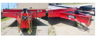
■ Longer drawbar & premium landing gear: Longest drawbar in the industry makes for better load distribution and easy handling. 1/2" safety chains are integral to the frame of the trailer, not welded in place. The two-speed landing gear has 50,000 lb. lift capacity and 70,000 lb. static capacity. The pintle eye adjusts to accomodate various heights using standard shop tools. There is ample room for chain and tool storage in the drawbar toolbox with lockable steel lid.
