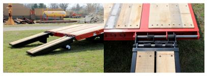
**Extra-long loading ramps with 72" beavertail at 8° slope:** Constructed from high-strength 50,000 psi minimum yield steel, these ramps are strong and durable yet lightweight for easy operation. Dual springs assist the operator lifting the ramps off the ground as well as off the deck. The ramps can be easily adjusted laterally to handle machines of various widths. Extra length reduces the climb angle for safer loading. These "E-Z Flip" ramps are standard oak-covered or optional ladder style.
