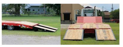
Simplified loading of machines with "E-Z Air" ramps and 65" long beavertail: The air operated wood-covered ramps are 38" wide by 84" long (96" with optional aluminum extensions). With the suspension air dumped, they provide a machinefriendly 13° load angle. The extra-long beavertail is also wood-covered and features a 7° incline. Full 1 <sup>3</sup>/<sub>4</sub>" thick air-dried oak deck is fastened to the trailer frame with carriage bolts and cupped washers.
