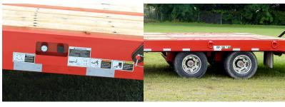
Heavy-duty air suspension and axles for a smooth and stable ride: Conveniently located controls operate both the air dump valve and the "E-Z Air" ramps for loading and unloading of machines. Optional aluminum disc wheels (outside only) are lightweight and look great. Both axles are equipped with spring parking brakes and a premium 4S/2M antilock braking system.
