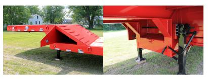
Long, flat gooseneck and tool boxes for storage: The full-width gooseneck provides a 10-foot long load area that is easily accessible from the trailer deck. The gooseneck is equipped with three toolboxes: a full-width one under the ramp, another one underneath the gooseneck frame and an oak-covered one over the kingpin. A heavy-duty two-speed landing gear set is standard equipment.
