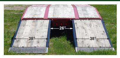
Available on the ROGERS TAG21XXL and TAG25XXL trailers, these newly designed air-operated ramps take the hard work out of loading and unloading your ROGERS trailer. At 38" wide by 96" long (with optional extensions), they are ideal for loading a wide variety of machines, from excavators and dozers to pavers and rollers.
