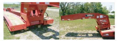
Exclusive "Croucher"® front with tapered beams gives an optimal approach angle. Concealed beam hooks won't damage low ground clearance equipment. Powerful, low operating pressure "No Foot"® self-lifting gooseneck saves time and effort by easily lifting the rated load on any terrain. The Scraperneck design lets equipment ride over the gooseneck to maximize load space.
