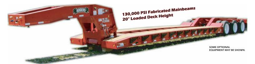
The ROGERS<sup>®</sup> **ULTIMA<sup>™</sup> CR50** - our high performance 50-ton capacity detachable gooseneck trailer. It features a low, tapered front end; the "No Foot"<sup>®</sup> self-lifting gooseneck; a "Bucket Pocket"and a ramp incline to the rear frame for additional load space. It's design of 1/2 load concentration, 50 tons in any 12'-0" of deck, means more load options for you.
