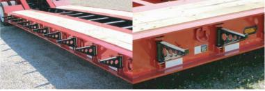
■ The unitized frame has fabricated main beams of 130,000 PSI steel the strongest in the industry. Full-width cross members on 24" centers for longer deck life. Full 1 3/4" air-dried oak decking installed with carriage bolts and cupped washers. Removable swinging side brackets widen the deck to 10'-6". Certified lashing D's with a 55° bend exceed today's load securement regulations.
