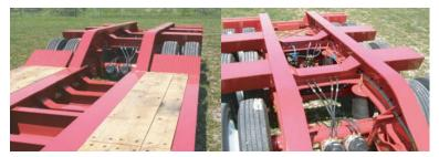
Last three (3) cross members of deck notched for a "Bucket Pocket". Convenient 30° ramp incline gives easy access to the rear frame, which has trunnion beams between wheels. Each axle has spring-loaded parking brakes for improved loading and unloading safety. The "Boom Trough" combines with the 20" loaded deck height for the industry's lowest transport height.
