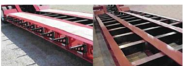
Unitized frame with mainbeams fabricated of 100,000 PSI steel. Heavy-duty, full-width cross members on 24" centers for longer deck life. Full 1 3/4" air-dried oak decking installed with carriage bolts and cupped washers for easy replacement. Optional heavy-duty swinging, removable cast side brackets widen the deck to 10'- 6". Tested and certified D-rings exceed today's load securement regulations.
