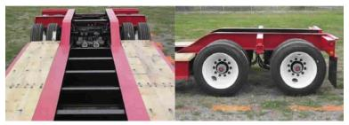
Lowered crossmembers in the rear frame provide extra space for excavator booms. "Lumber to the tires" yields an extra foot of deck space. Light-weight trunnion beams are used to tie-down loads. Spring loaded parking brakes provide improved loading and unloading safety.
