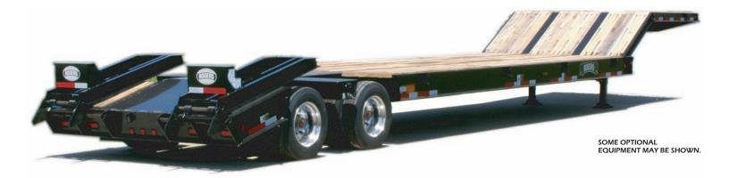
The ROGERS® **FIXED GOOSENECK MH25** – a "carry all" trailer with the combined conveniences of a rear loading style, a spacious level deck, and sloped access to the full-width gooseneck. It is a gooseneck style that can hold machine equipment or a cargo load. This 25-ton Machinery Hauler has the streamline dependability to provide trouble-free service.
