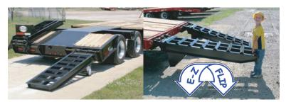
Rear frame has trunnions between wheels and LED lights package. The 14° sloped beavertail has "E-Z Flip" loading ramps constructed of high strength steel, yet are light enough for easy operation with dual springs to assist lifting. Plus these ramps have easy lateral adjustments to handle machines of various widths. Standard ramps are oakcovered: photo shows optional ladder style.
