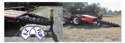
■ Extra-long loading ramps with 14° beavertail. Constructed from high strength steel, these ramps are heavy-duty yet light enough for easy operation. Dual springs lift the ramps off the ground as well as off the deck. The ramps have easy lateral adjustment to allow loading machines of various widths. The E-Z Flip ramps are available in standard oak covered !or optional ladder style.
