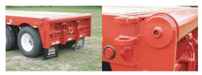
■ The rear design of the trailer has dozer push bars and a tow ring. It features a heavy-duty 8" diameter "tail roller" built with bushings for durability. Other standard features are (18) pipe pockets, removable mud flaps, and 1 3/4" air-dried oak decking installed with carriage bolts and cupped washers.
