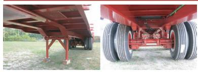
Heavy-duty main beams and side channels with deep cross members combine to make a strong and durable trailer frame. The heavy-duty undercarriage includes flip-leg landing gear and single-point, two-spring suspension. Both axles have spring parking brakes and a premium 4S/2M anti-lock braking system.
