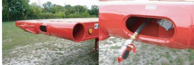
The OF40L trailer has a rounded front designed with an attachment for winch lifting. It has a pair of recessed air line glad hands that are retractable so cleaning off dirt and mud is easier.
