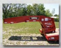
The powerful "No Foot®' self-lifting detachable gooseneck operates with low pressure and easily lifts the rated load on any terrain.
