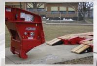
A pair of hooks at front of main frame interlocks with the matching hooks on the bottom of the gooseneck.
