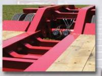
The "bucket pocket" has lowered cross members in the rear deck to tuck an excavator's bucket. Bridge ramps are reinforced tread plate at 30° slope for equipment to load on the rear frame.
