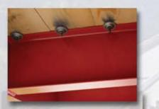
The platform deck has an open center and 13/4" air-dried oak installed with carriage deck bolts and cupped washers. The deck is 2" oak on the 60-ton.
