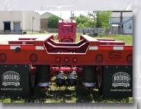
The "boom trough" has notched cross beams in the rear frame opening for lowering an excavator's boom to improve overhead clearance.
