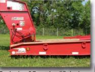
Exclusive "Croucher®" design has main beams tapered top and bottom and concealed beam hooks for easy front-end loading.
